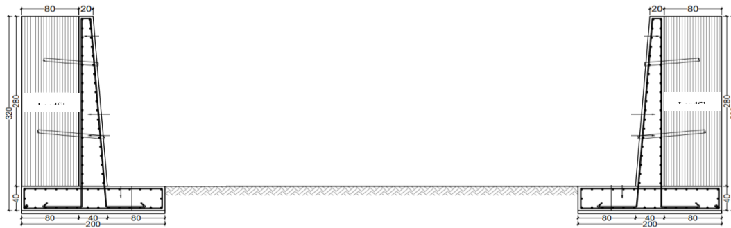
Figure 4. Alternative 2 (Concrete Sheet pile)
