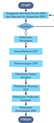
Gambar 1. Flowchart Pekerjaan Steel Sheet Pile (SSP)
